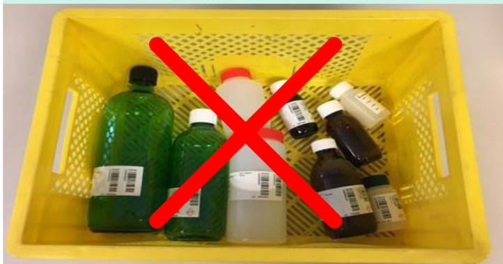
**Bottles firmly placed in crate, do not protrude above edge**
